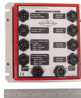
The Amerex Vehicle SafetyNet Driver Panel includes the most common features required for vehicle fire protection and gas detection system. The Driver Panel is virtually identical to the proven AMGaDS III Driver Panel design. The SafetyNet Driver provides a connecting point for fire suppression & gas detection field wiring.
